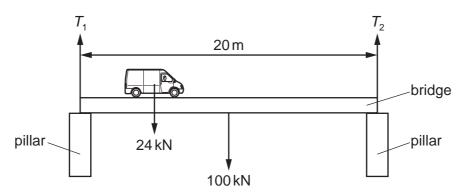
The pillars exert forces  $T_1$  and  $T_2$  on the ends of the bridge.
